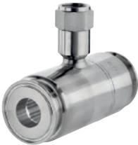
In-line seals are integrated directly into the process line. They are less temperature-sensitive than diaphragm seals and are particularly suitable for applications, which are absolutely free of dead space, with circulating, highly viscous media, with media tending to swirl and for applications with frequent changes of the medium.
