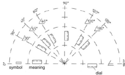
The medium shall be able to drain. Please do not install pressure gauge and chemical seal upside down.
